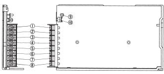
1V1 Output 2G1(V1)GND 3V2 Output 4G1(V2)GND 5NC ⑥Frame ground
