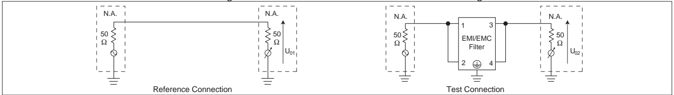
Fig.3.2 Common mode attenuation measurement diagram
