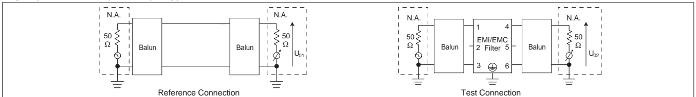
Fig.3.3 Differential mode attenuation measurement diagram
