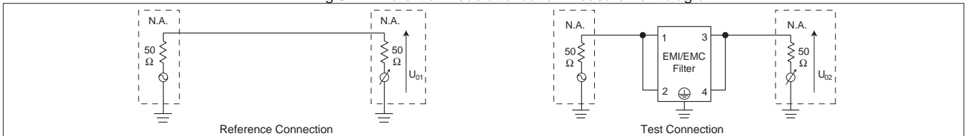
Fig.3.2 Common mode attenuation measurement diagram
