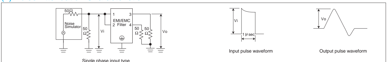
Fig.3.7 Pulse attenuation measurement diagram
