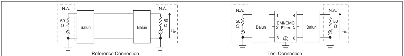
Fig.3.3 Differential mode attenuation measurement diagram
