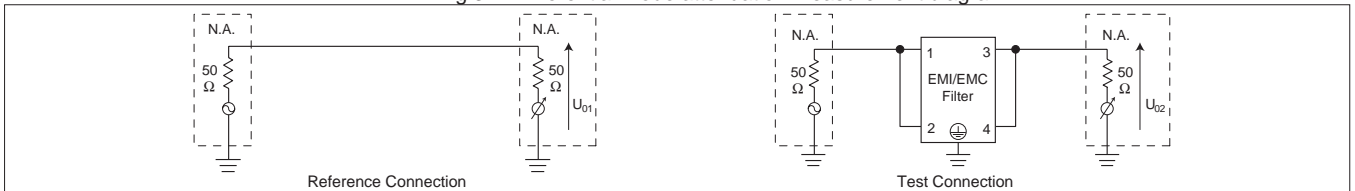
Fig.3.2 Common mode attenuation measurement diagram
