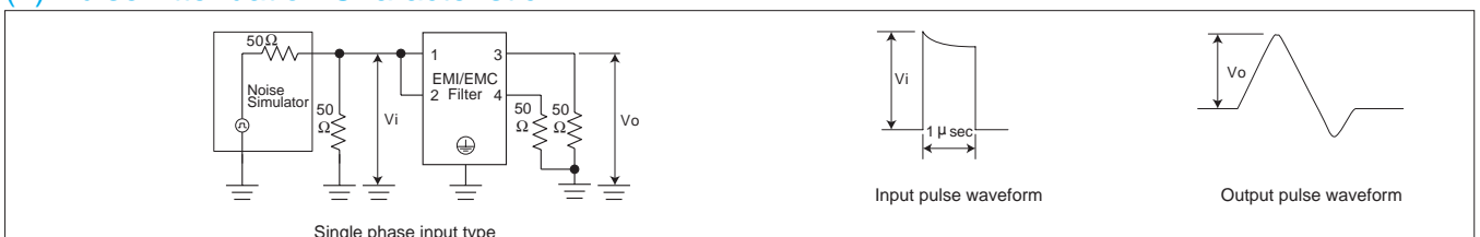
Fig.3.7 Pulse attenuation measurement diagram
