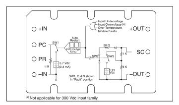
Figure 2 — PC/SC module alarm logic.
