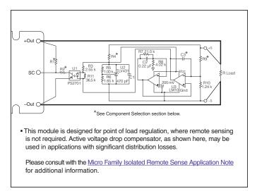
Figure 12 — Voltage drop compensation.
