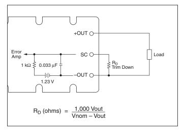
Figure 7 — Output voltage trim down circuit.
