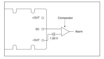
*Figure 6* — *Secondary side on-state indicator.*
