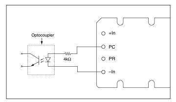
Figure 5 — Isolated on-state indicator.
