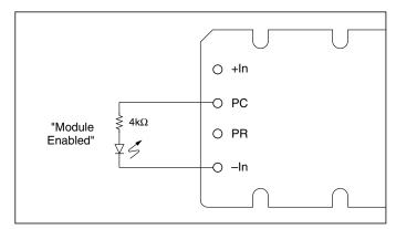
Figure 3 — LED on-state indicator.
