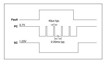
*Figure 4* — *PC/SC module alarm timing.*
