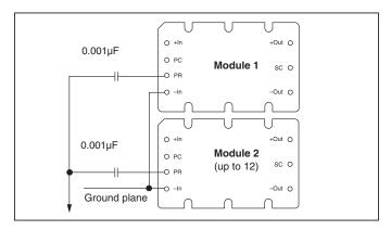
*Figure 10* — *AC coupled single-wire interface.*
