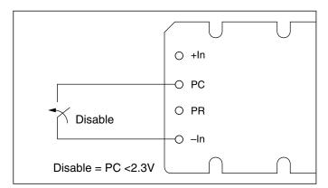
Figure 1 — Module enable / disable.
