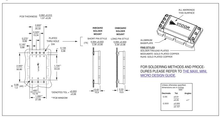
Figure 14 — PCB mounting specifications
