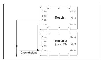
*Figure 9* — *DC coupled single-wire interface.*
